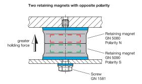
If two retaining magnets with opposite polarity are combined, an increased holding force is achieved.
